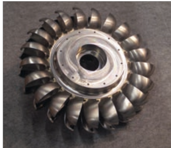
Pelton wheels work on higher gradients
