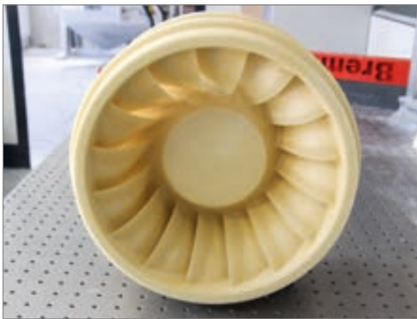
A model of the impeller made from a meltable material, created using 3D printing
