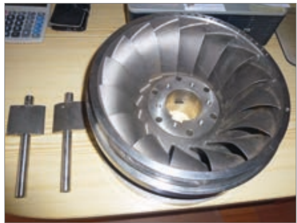
Stainless steel castings of the “heart” of the turbine
